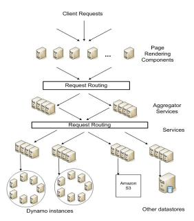
Figure 1: Service-oriented architecture of Amazon's platform
